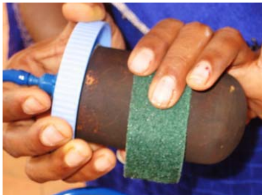
Figure 2.7 Scrubbing the ceramic element with the included scrub pad (van der Ven-TWF, 2008)
