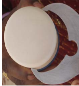
Figure 2.8 Measuring the ceramic element using the end-of-life gauge (BWN-IU, 2008)
