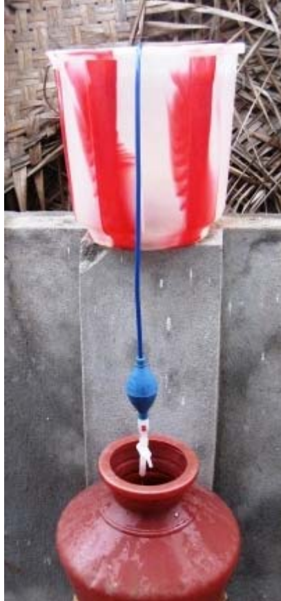
Figure 2.6 Tube, bulb and tap of siphon filter (van der Ven-TWF, 2008)
